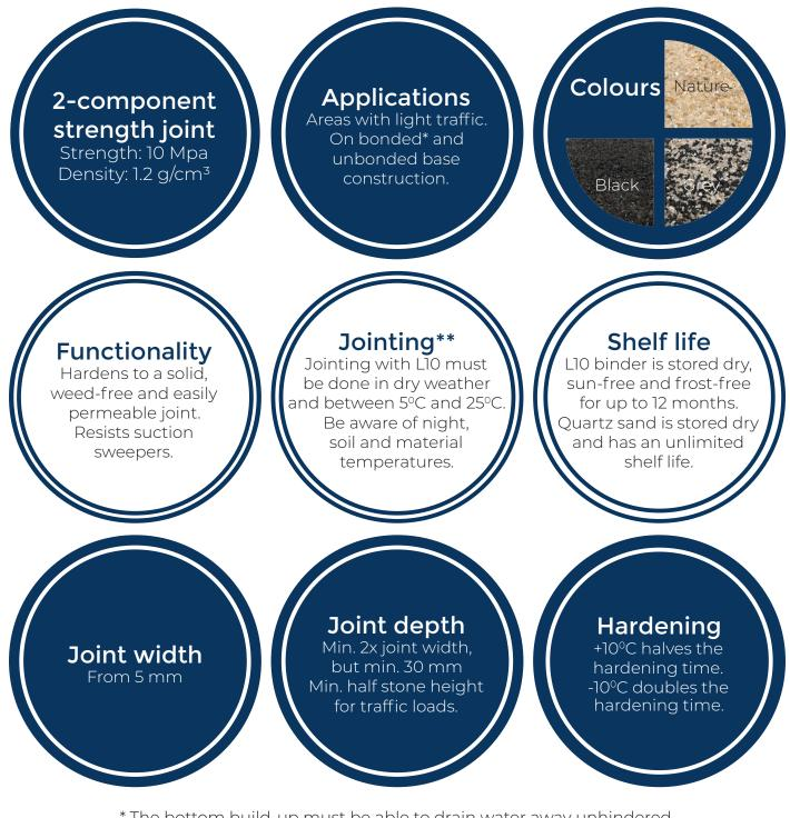
\* The bottom build-up must be able to drain water away unhindered. If an expansion joint or similar is used, it must be 1:1 in the pavement.
